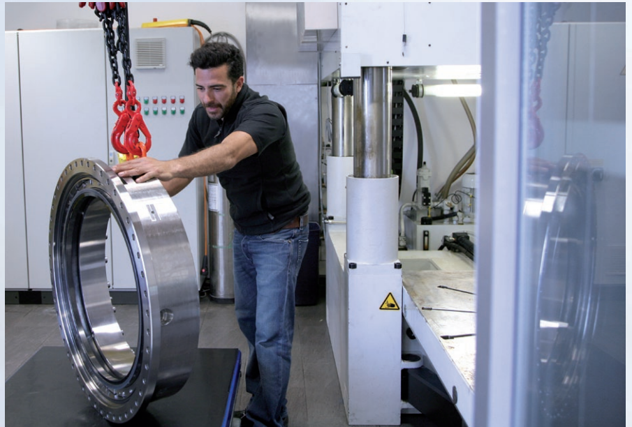
The fully split mechanical seal VGH300 for a shaft diameter of 550 mm (21.65") being prepared for the test run.
